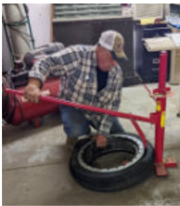
Gary breaking the bead on the F-84 main tire (K. Drewelow photo)
